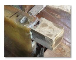
With the engine bed marked, reinforcing "backers" were then epoxied into place. Given the geometry of the hull, it would be impossible to use regular machine bolts to secure the engine
