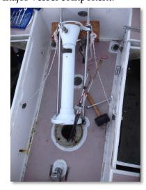
cables could be pulled out. The new cables were then snaked up the column and secured with a screw to hold the cable clamp to the inside of the column.
