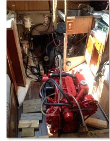
coupling in the drive train increased this difference by a little over 3 inches. Also worth noting (as it becomes significant in the next paragraph), is that the alternator is located on the port side of the motor, opposite that of the Atomic Four.
