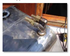
Part of the conversion from the Atomic Four engine is that the new motor has fuel injection instead of carburation. A common practice with injectors is to pump more fuel
