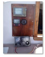
location. The autopilot controller and the old tachometer were then removed and a jigsaw was used to create the necessary opening. The new panel was inserted into the hole and secured with four screws and the wiring harness was snaked down into the engine compartment.
