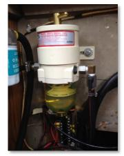
mounted in an easily accessible place so that it can be checked, drained and changed whenever needed.
