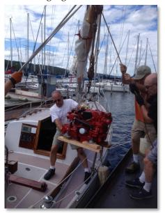
While four people could lift the engine on its pallet on dry land, doing so to transfer it to a boat floating in a slip was not practical, so step one was to place the motor on the dock where it could be picked up from the boat. The slip used by our marina travel lift was chosen
